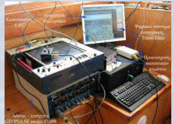
Geopulse Transceiver/Receiver Triton Elics Digital Acquisition system
