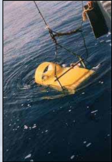
3.5 kHz ORE Pinger with 4 and 9 transducers
