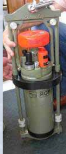
Multi-parameter seawater sensor and current meter Aanderaa RCM9 MK II.
