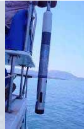
Multi-parameter seawater sensor and current meter Aanderaa RCM9 MK II.
