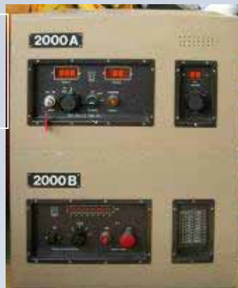
Geopulse Transceiver/Receiver Triton Elics Digital Acquisition system
