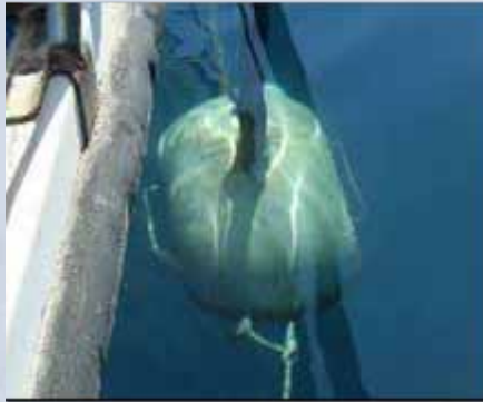
3.5 kHz ORE Pinger with 4 and 9 transducers
