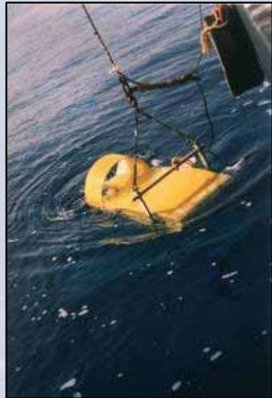
3.5 kHz ORE Pinger with 4 and 9 transducers
