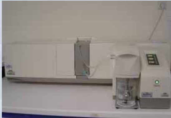
particle size analyzer (MasterSizer 2000)
